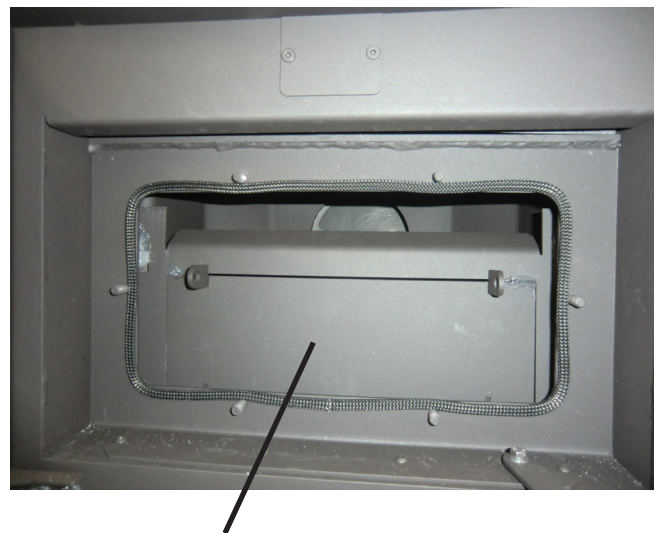
Fig. 5 Separating wall water-heat exchanger
